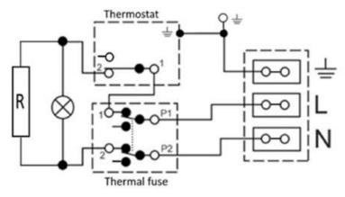
Heating unit 3.3 kW and 6,6 kW
