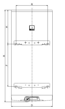
Upper and lower Hinge 200 I 4 anchoring screws Dimensiions 450mm and F check before drilling
