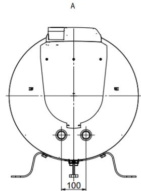
Upper suspension + detent support (rectifying screw)
