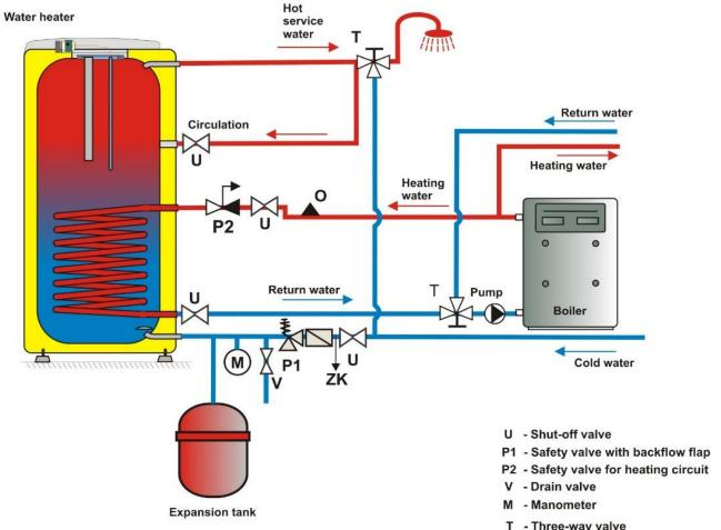
\* Use of expansion tank is not a prerequisite of correct connection but just a possible design variant
