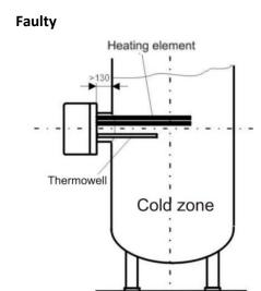
Too long flange welded too high. Thermowell under the heating element.
