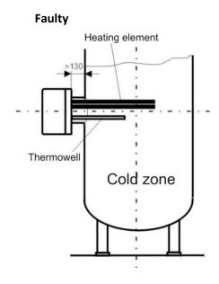
Too long flange welded too high. Thermowell under the heating element.
