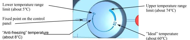
**Notice:** Adjusting the thermostat selector at the left backstop does not mean permanent shutoff of the heating element. When the heater is in use without blocking the daily rate, we do not recommend the temperature to be set above  $65^{\circ}$ C. The maximum value to select is "60".
